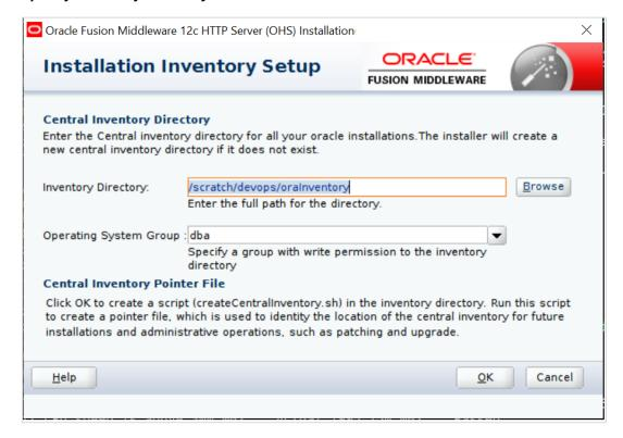
This screen appears for UNIX systems only; if this is your first Oracle installation on this host, you must specify the location of the inventory directory. This inventory directory is used by the installer to keep track of all Oracle products installed on the computer. The default inventory location is USER\_HOME/oralnventory.
